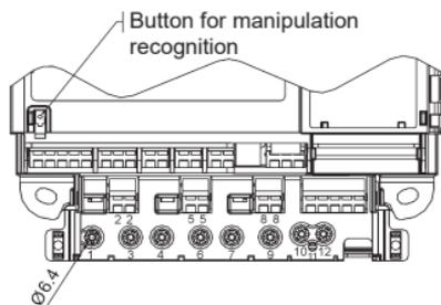
For testing the device, the voltage paths are interrupted by a path separator.
