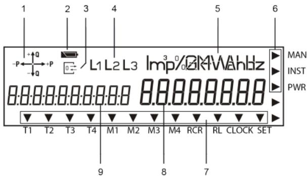
1. The **operation indicator** shows the energy direction currently measured by the meter (supply/drawing of active power, inductive/capacitive reactive power). If there is a consumer current flowing, the energy direction arrows show in which quadrant the value is measured. E.g.:
