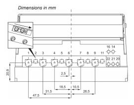
For test purposes the voltage path can be separated from the current path. For this, the voltage slide of all 3 phases in the terminal block must be opened (see detail). To do this, loosen both screws and push the voltage slide to the right. Afterwards, tighten the screws with the permitted torque according to table 1.
