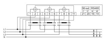
4-wire version, connected to current- and voltage transformer
